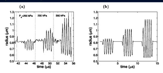
FIG. 8. (a) Experimental recordings of a BR14 bubble response to repeated 2 MHz pulses separated by 60 ms, with an increasing acoustic pressure. (b) Simulation with the same acoustic pressures. The fitted shell parameters are  $R_{\rm buckling} = R_0 = 0.82 \ \mu {\rm m}$ ,  $\chi = 1 \ {\rm N/m}$ ,  $\kappa_s = 7.2 \times 10^{-9} \ {\rm N}$ , while the critical break-up is  $\sigma_{\rm break-up} = 0.13 \ {\rm N/m}$ .
