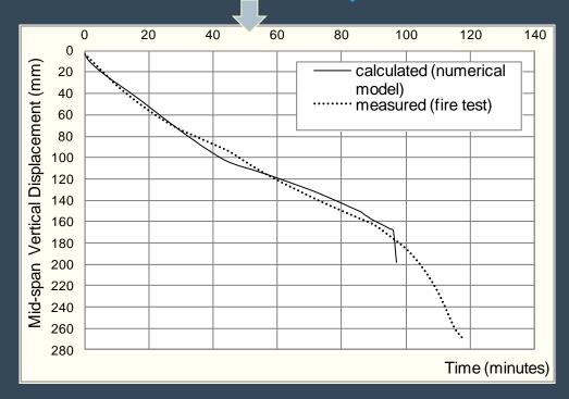
2. Thermo-mechanical modeling of composite slabs with thinwalled steel sheeting submitted to fire
