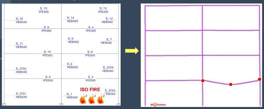
Fire resistance: 23 mins. Finally the system fails???????
