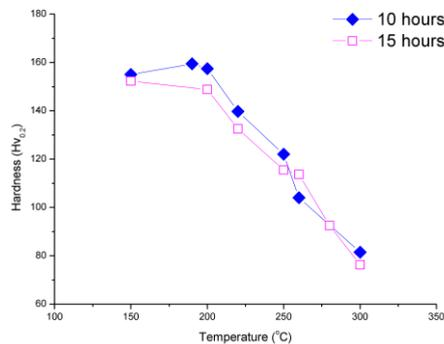
Fig. 1. Overaging curves of 2024 T3 aluminum alloy showing variation of hardness with temperature
