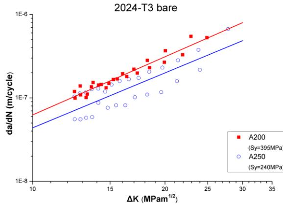
Fig. 8. Fatigue crack growth rates versus stress intensity factor range ( $da/dN-\Delta K$ ) in bare A200 and A250 materials
