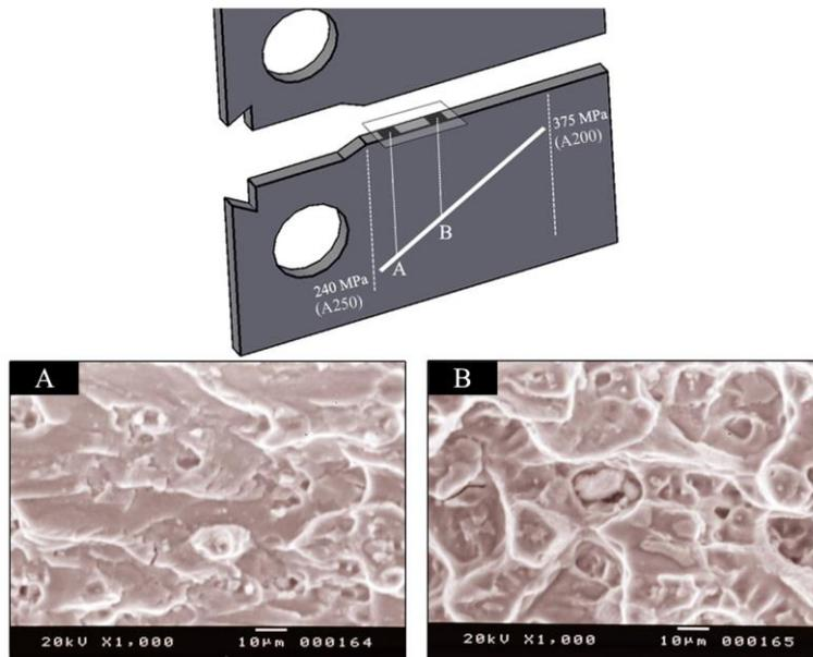
Fig. 9. SEM micrographs of specimen with increasing yield strength profile showing fracture surface characteristics during FCG at range a)  $\Delta K=11 \text{ MPam}^{1/2}$  b)  $\Delta K=20 \text{ MPam}^{1/2}$
