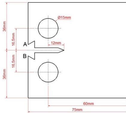
Fig. 4. C(T) specimen configuration according to ASTM E 647-00
