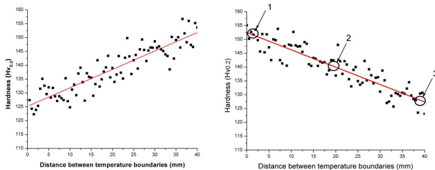
Fig. 2. Hardness profiles of specimens after heat treatment (a) linear hardness increase with distance (b) linear hardness decrease with distance
