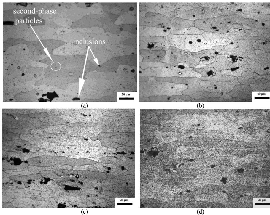
Fig. 3. Microstructure of (a) 2024 material in T3 state; and materials subjected to artificial aging (b) position 1; (c) position 2; (d) position 3 of Fig.2b
