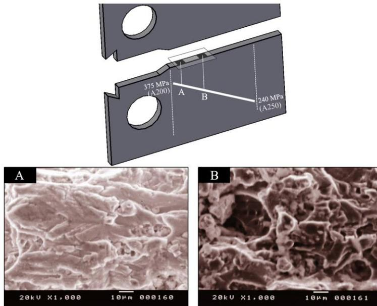
Fig. 10. SEM micrographs of specimen with decreasing yield strength profile showing fracture surface characteristics during FCG at range a)  $\Delta K=11 \text{ MPam}^{1/2}$  b)  $\Delta K=20 \text{ MPam}^{1/2}$
