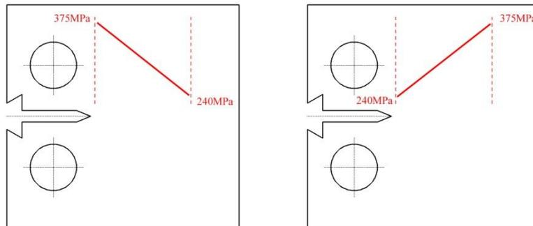
Fig. 5. C(T) specimen with (a) decreasing; and (b) increasing strength gradient boundaries in front of notch tip resulting from heat treatment
