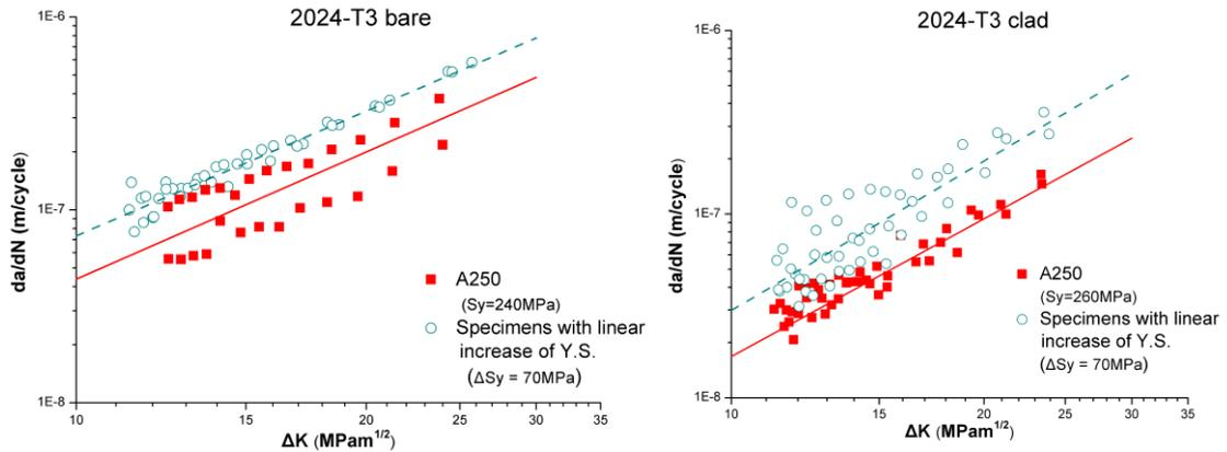
Fig. 6. Fatigue crack growth rates versus stress intensity factor range ( $da/dN-\Delta K$ ) in A250 and material with increasing yield strength with regard to the crack tip (a) bare 2024-T3; (b) clad 2024-T3
