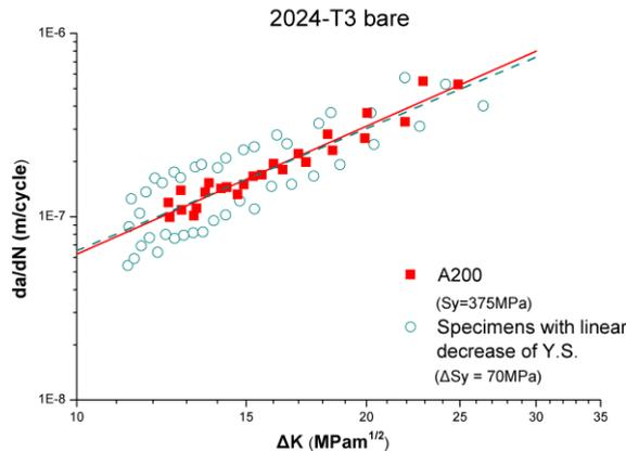
Fig. 7. Fatigue crack growth rates versus stress intensity factor range ( $da/dN-\Delta K$ ) in bare A200 and material with decreasing yield strength with regard to the crack tip
