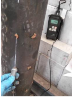
Figure 11: Steel pipe specimens and thickness measurements via ultrasonic device.
