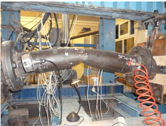
Figure 15: Dented specimen SP5d during cyclic 4-point bending.
