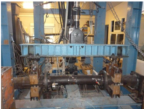
Figure 7: Four-point bending experimental set-up.
