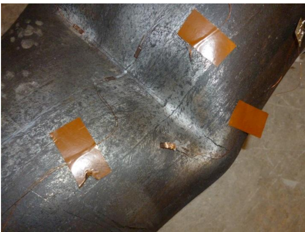
Figure 5: Instrumentation of pipe specimen.
