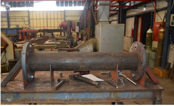
Figure 2: 6-inch X52 pipe specimens.
