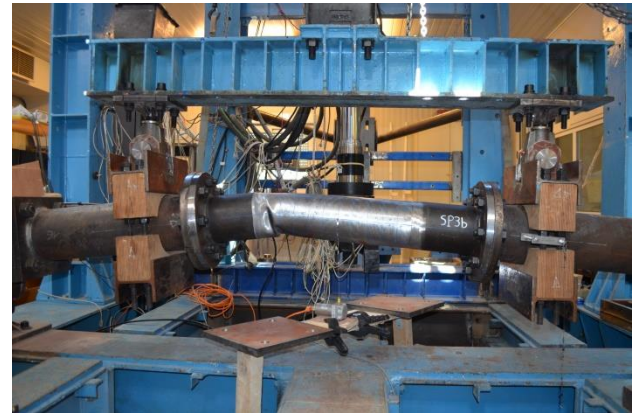
Figure 3: Four-point bending experimental set-up.
