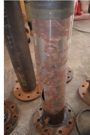
Figure 21: Rupture of SP8b specimen, away from the buckled area
