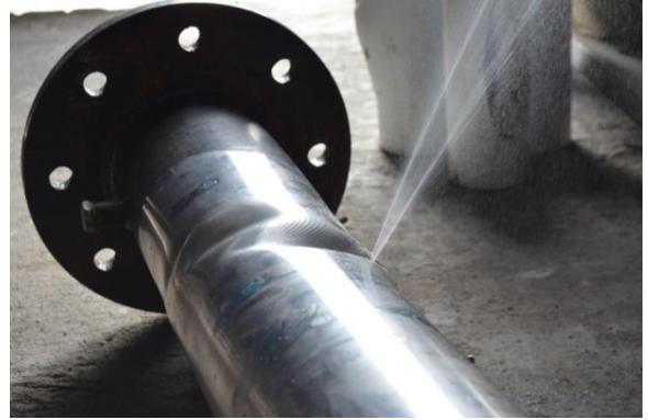
Figure 20: Leakage of specimen SP7b due to cyclic internal pressure; wall rupture location at the buckle location.
