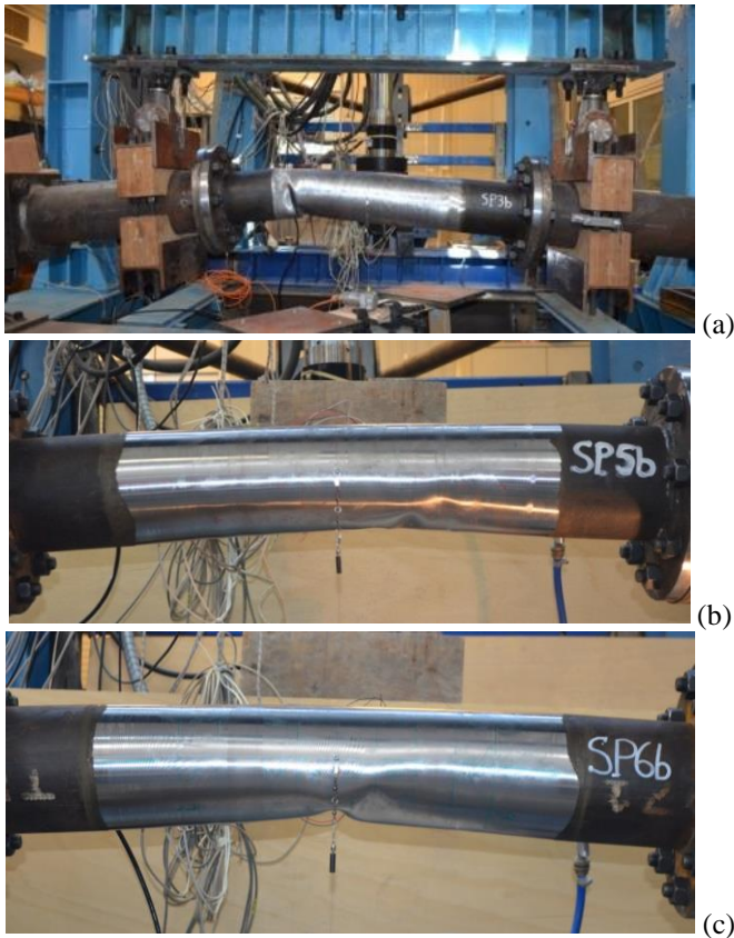
Figure 15: Buckled specimens (a) SP3b, (b) SP5b and (c) SP6b buckled specimens.
