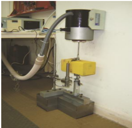
Figure 4.2: Experimental set up for measuring the support stiffness and damping parameters.
