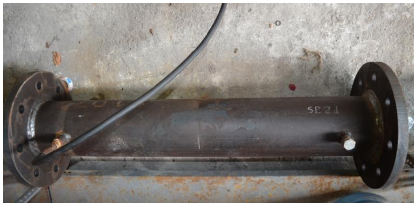
Figure 3-25: Pressure application on specimens \text{Ø}168.3/4.78 .
