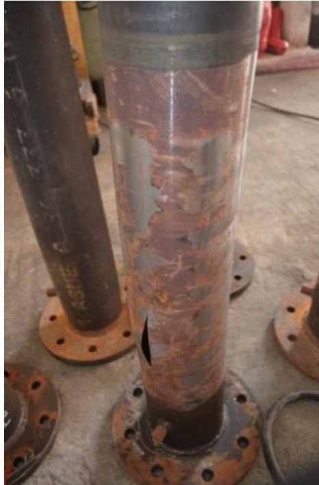
Figure 3-60: Rupture of SP8b specimen, away from the buckled area
