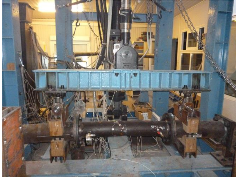
Figure 3-19: Four-point bending experimental set-up.
