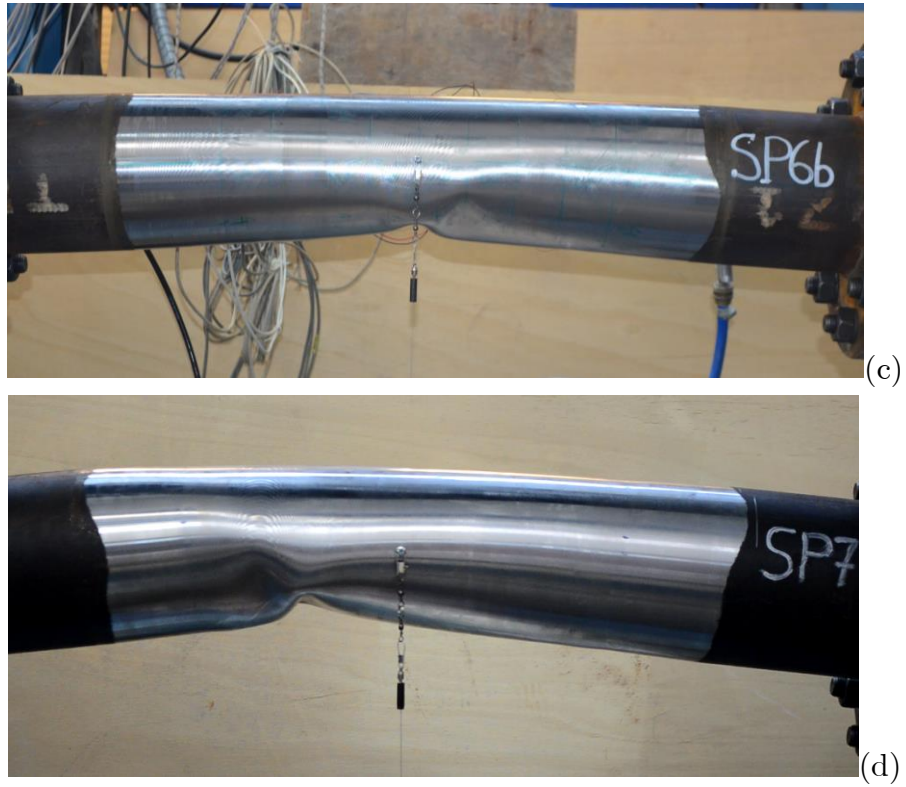
Figure 3-51: Side views of buckled specimens (a) SP3b, (b) SP5b, (c) SP6b and (d) SP7b buckled specimens.
