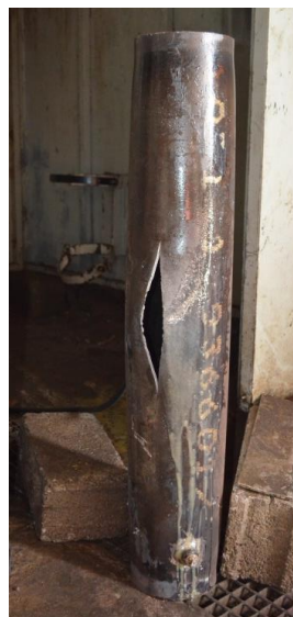
Figure 3-63: Rupture of perfect \text{Ø} 168.3/4.78 specimen
