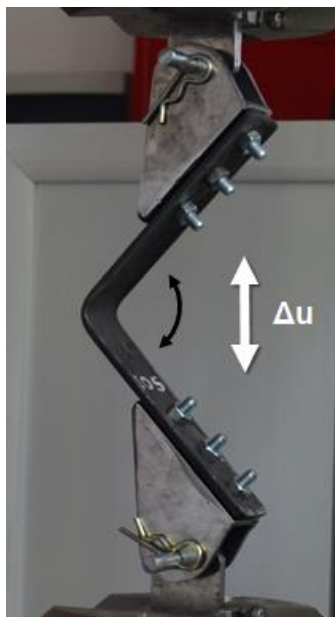
Figure 5-3: Loading and test configuration of strip specimens
