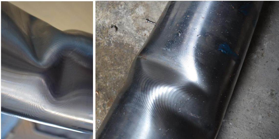
Figure 3-61: Buckled specimen SP7b: (a) buckle region prior to pressure application and (b) after cyclic internal pressure
