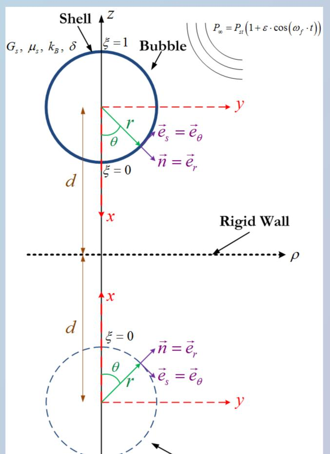
Schematic representation of a coated microbubble near a rigid boundary depicting the global coordinate system  $(\varrho, z)$ , the local coordinate system  $(r, \theta)$ , the initial distance (d) between bubble and wall, the disturbance of the pressure field, where  $\epsilon$  is the amplitude of the latter and  $\xi$  is the Lagrangian marker on the interface
